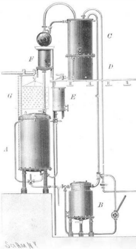
EGROT APPARATUS FOR THE EXTRACTION OF PERFUMES BY VOLATILE SOLVENTS.
